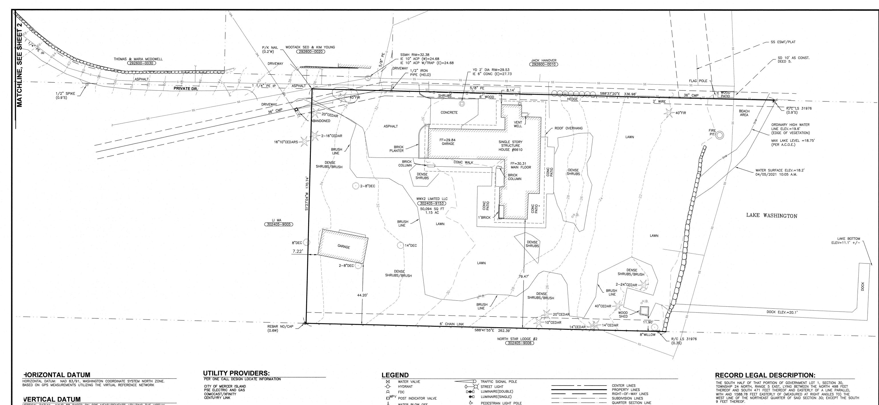
VERTICAL DATUM: NAVD 88 BASED ON GPS MEASUREMENTS UTILIZING THE VIRTUAL REFERENCE NETWORK AND GEOID 2012A MODEL.
